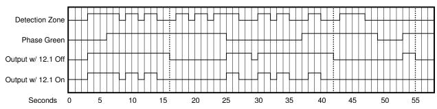
This example assumes an extension time of 2 seconds. The dotted lines show where disconnect would occur. Phase Green is the state of the light (actual Phase Green Input is inverted).
