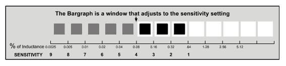
The bargraph, below, has the same vehicle in the loop zone causing the same inductance change as above. Since the sensitivity setting was increased to Level 7, six segments are now displayed. If the bargraph displays 5 or 6 segments for a vehicle in the loop and motorcycles are not a concern, the sensitivity has been set to the proper range.
