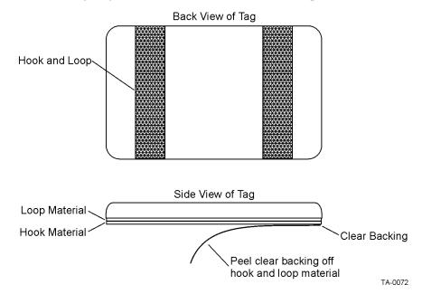
Figure 3-21 Hook-and-Loop Material on Interior Tag
