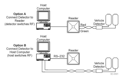
Figure 8-8 Encompass 4 Reader RF Control Options
