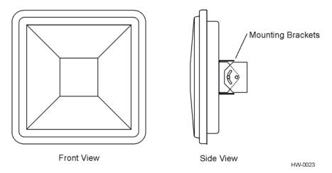
Figure 1-1 Encompass 4 Reader System Front and Side Views
