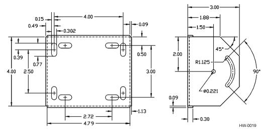
Figure 4-6 Pole-Mount Bracket Assembly
