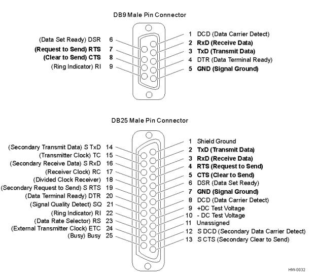
Figure C-1 DB9 and DB25 Connector Pin Assignments for Signal to Host
