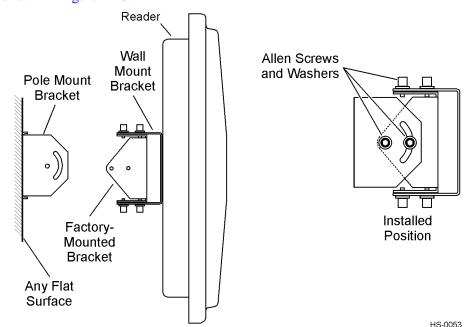
9. Mount the Encompass 4 Reader to the pole-mount bracket using Allen screws, as shown in Figure 4-13.
