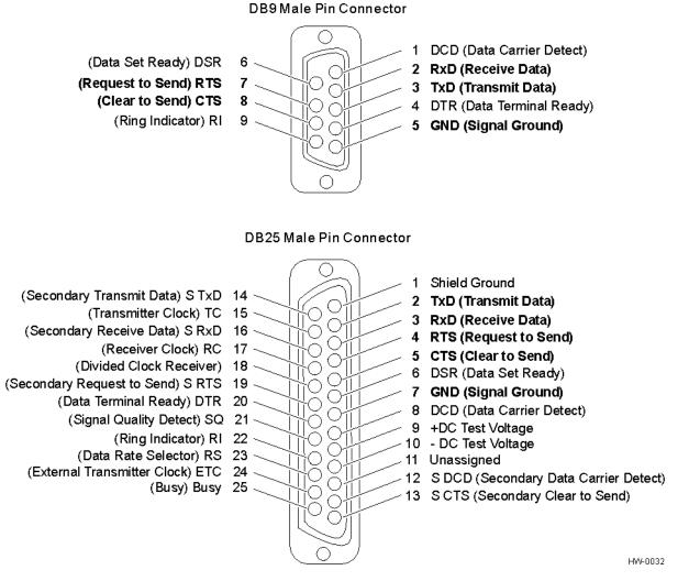
Figure 4-3 Pin Assignments for Signal to Host Connectors
