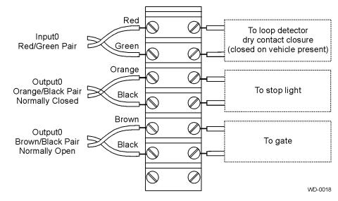
Figure 4-16 Sample Circuit Connections
