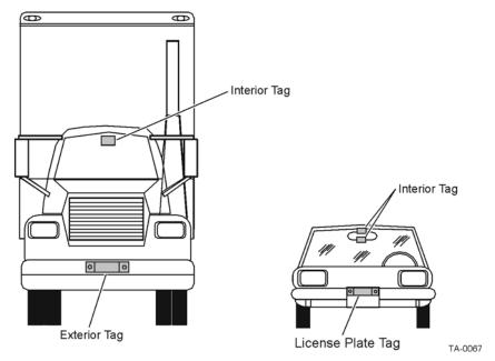
Figure 2-5 Typical Tag Positions Used with Overhead Reader
