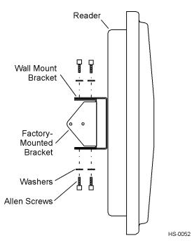
Figure 4-11 Factory-Mounted Bracket Attached to Wall Mount Bracket
