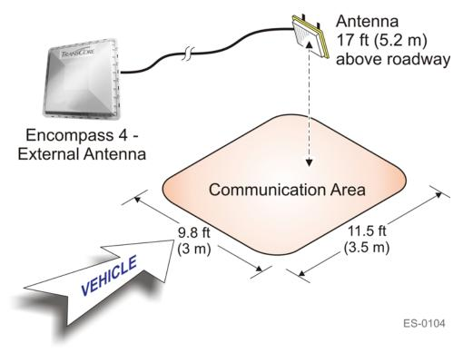
Figure 4-15 Encompass 4 Reader Installation with Overhead Antenna
