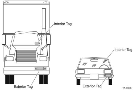
If the Encompass 4 Reader is installed on a pole or wall to the left of the vehicle, optimal tag position is on the left side of the vehicle as illustrated in Figure 2-3.
