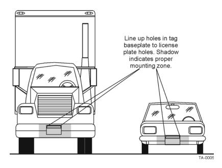
Figure 3-13 Correct Mounting Location for LPT
