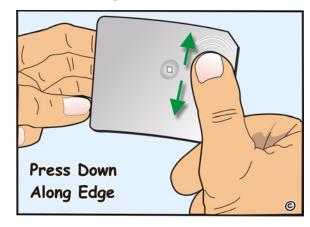
Figure 3-9 Applying eGo Plus Sticker Tag to Windshield
