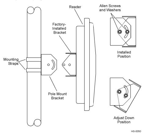
that the Encompass 4 Reader can be adjusted up or down, but not so slightly the mounting assembly slips.
