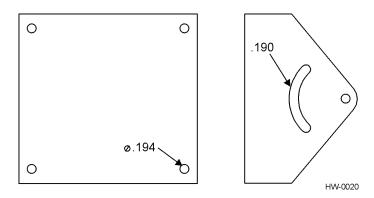
Figure 4-9 Wall Mount Bracket Accessory (part number 54-1620-001)
