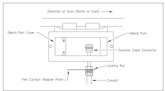
**22** Put the scanner cable connector through the northmost or eastmost round hole in the side of the mount.
