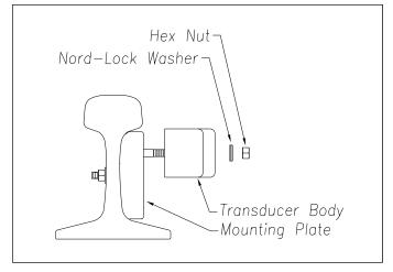
The installed transducer body should be 1-9/16 inches (3.97 centimeters) below the top of the rail <u>and</u> parallel to it. You can meet this requirement by using the transducer height bracket on the bottom of the alignment fixture.
