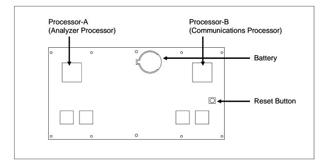
The figure below shows a Processor board (2300-100).
