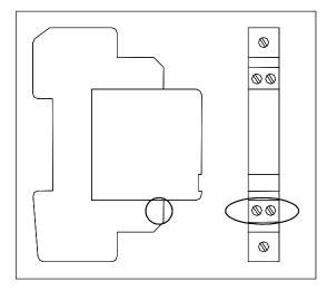
Each UTB is mounted vertically on a DIN rail. Shown to the left are two views of the same UTB.
