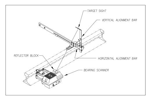
Shown below is alignment of a type2 bearing scanner.
