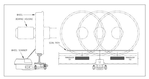
The **<u>type3</u>** wheel scanners are aligned to scan about 4 inches (10.2 centimeters) above the rail.
