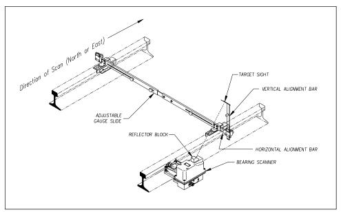
**12** Extend the horizontal alignment bar to 7-1/4 inches  $\pm$  1/4 inch on the scale.
