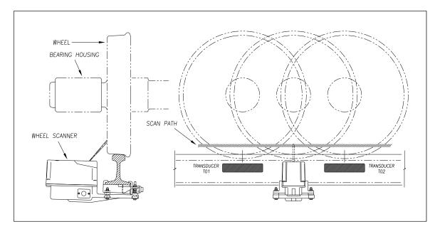
The SmartScanIS checks for hotwheels during the scanning process. Scan timing is controlled the same as for the bearing scanners.
