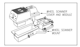
The figure below shows the major parts of a type3 wheel scanner.
