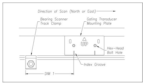
Note that the hole (on top of the bearing scanner cover) faces north or east. Note further that the gating transducers are mounted on the same side as where the bearing scanner is "looking."
