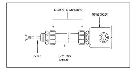
One end of the transducer cable comes attached to the transducer. The other end has two wires protruding from the conduit. These wires are black and white. They attach to a surge protector located on the surge-protection panel. There is one surge protector assigned to transducer TO1 and another to transducer TO2. These surge protectors protect the SmartScanIS from transients and surges, which can be induced onto external wiring by lightning.
