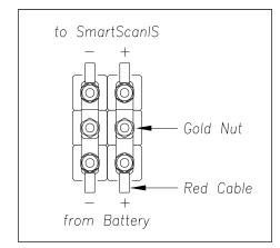
3 Cut a red-black 10 AWG 2-conductor wire to fit between the battery and the battery block.
