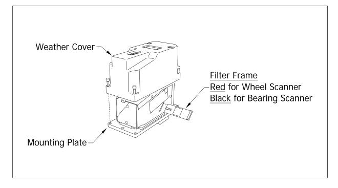
The figure below shows a <u>type2</u> wheel scanner mount (2100-701). Though <u>not</u> recommended, this mount can also be used for <u>type3</u> wheel scanners. However, this guide does <u>not</u> cover the use of this mount for <u>type3</u> wheel scanners.
