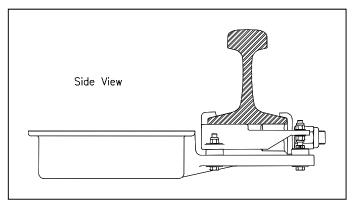
On the side of the mount are a large hole and <u>two</u> socket-head-cap screws. The longest screw is holding a ground lug and an internal-tooth washer.
