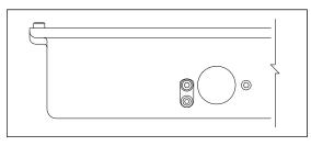
For the **type3** wheel scanner, the large hole is on the side of the mount (2500-401) farthest from the track. Some of these scanners have two ground lugs, as shown below.
