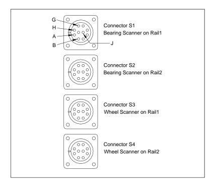
Connectors S1 through S4 on Scanner Interface board each have the same printout. The table below shows this pinout.
