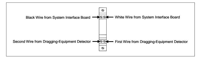
Correct polarity <u>need not be</u> observed when connecting the wires from the detector. One wire from the detector should be connected directly below the existing white wire at row two of the UTB, and the other wire should be connected directly below the existing black wire at row two of the UTB.
