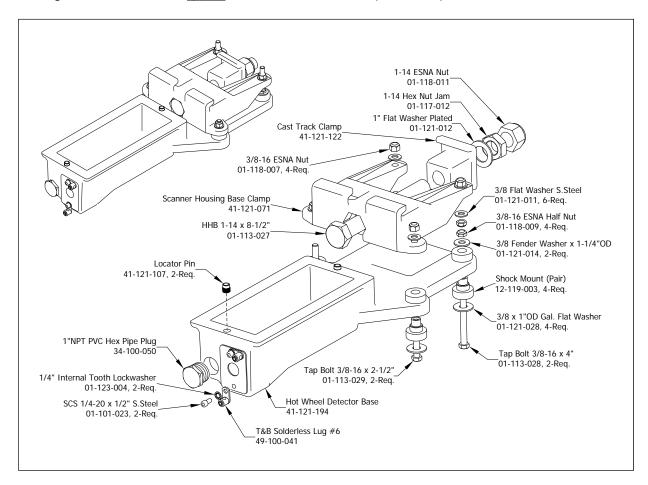
The figure below shows a type3 wheel scanner mount (2500-401).
