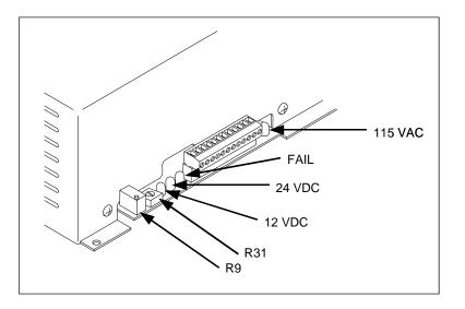
To adjust the battery float voltage:
