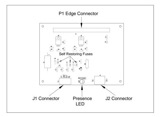
The 2200-500 SOTC Interface board has one LED. If everything is functioning properly, a lit LED indicates that a train is present. An unlit LED indicates that no train is present. While in calibration mode, the LED flashes until calibration is complete. Also, the 28-pin edge connector connects the 2150-500 SOTC Interface board to the 2300-528 Zepic III board.
