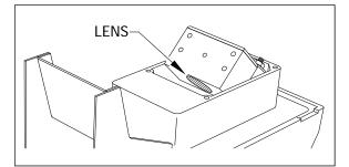
**10** Using a <u>soft dry cloth</u>, remove any accumulated dirt or grit.
