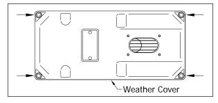
4 Remove the <u>weather cover</u> from its mounting plate.
