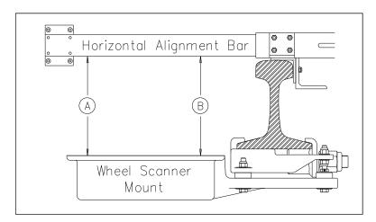
Alignment must be performed when a new scanner is installed. Thereafter, unless the scanner is damaged, it is unlikely that alignment will change once it has been set.
