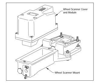
To replace a type2/type3 wheel scanner cover-and-module assembly:
