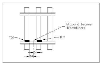
Use a permanent marker, magic marker, lumber crayon, or paint pen to mark the rail. Don't use a file or punch to mark the rail.
