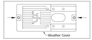
The **<u>type3</u>** bearing scanner has six. <u>Four</u> that attach the weather cover to the mounting plate and <u>two</u> that attach the mounting plate to the mount.
