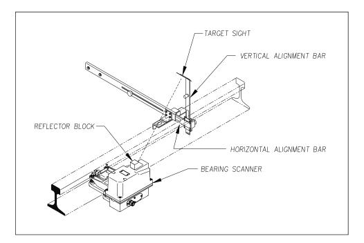
To align **type2/type3** wheel scanners, you use the horizontal alignment bar of the fixture. Alignment is done by measuring from the bottom of the extended bar to the top of both ends of the scanner mount. When both measurements are the same, alignment is correct. That is, as shown below, when distance **A** is <u>equal to</u> distance **B**, alignment is correct.
