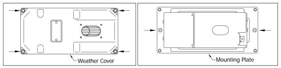
6 Separate the bearing scanner cover-and-module assembly from its mount.
