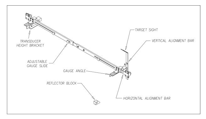
The figure below shows an assembled alignment fixture (2066-000).
