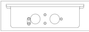
On the side of the mount are two large holes and <u>four</u> socket-head-cap screws. The longest screw is holding a ground lug and an internal-tooth washer.
