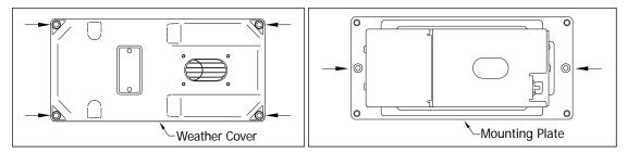
6 Separate the wheel scanner cover-and-module assembly from its mount.
