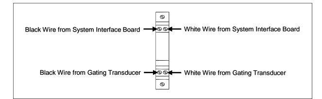
**Observe correct polarity** when you connect the wires from the transducers. The polarity is correct when the transducer's white wire is connected directly under the existing white wire at row two of the UTB, and the transducer's black wire is connected directly under the existing black wire at row two of the UTB. Connect **TO1** first and **TO2** second. **TO1** is the gating transducer <u>closest to</u> the bearing scanner. **TO2** is the one <u>farthest from</u> the bearing scanner.
