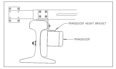
The fixture should be snug against the top and gauge of both rails. This may be impossible if the transducer body is less than 1-9/16 inches (3.97 centimeters) below the top of the rail <u>or</u> if the transducer body is not parallel to the top of the rail.
