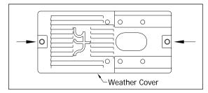
The **<u>type3</u>** wheel scanner has six. <u>Four</u> that attach the weather cover to the mounting plate and <u>two</u> that attach the mounting plate to the mount.
