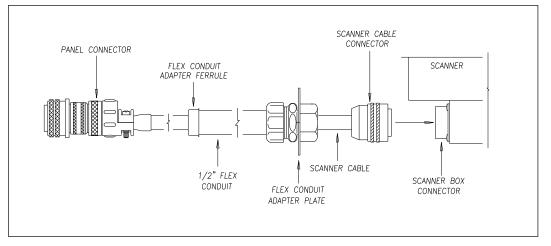
**Single-track sites** have two 65-foot (19.8-meter) wheel scanner cables. **Double-track sites** have two 65-foot wheel scanner cables for the track <u>closest</u> to the bungalow. For the track <u>farthest</u> from the bungalow, they have either two 85-foot (25.9-meter) <u>or</u> two 100-foot (30.5-meter) wheel scanner cables.
