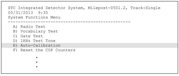
The **Auto-Calibration option** is used to calibrate the system's pyrometer interface circuitry.
