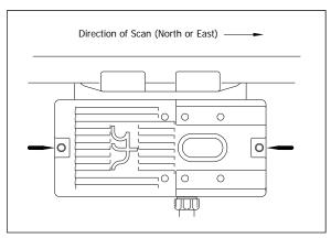
**b** Using the T-handle 1/4-inch hex-wrench, uniformly tighten the <u>two</u> socket-head-cap screws.
