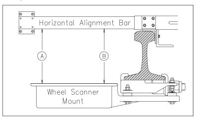
When both measurements are the same, alignment is correct. That is, as shown above, when distance **A** is <u>equal to</u> distance **B**, alignment is correct.
