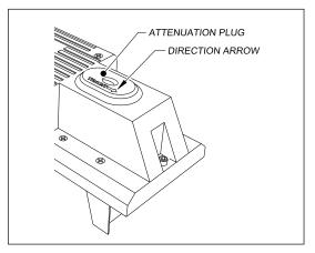
11 If you are calibrating <u>type3</u> wheel scanners, be sure that a <u>black</u> filter frame is still installed <u>in each scanner</u>.
