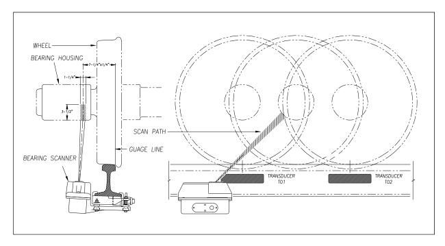
The **type3** bearing scanners are aligned to scan the bottom 3.5 inches (8.9 centimeters) of the bearing housing, about 7.25 inches (18.4 centimeters) from the gauge line.
