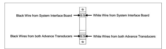
**Observe correct polarity** when you connect the wires from the transducers. The polarity is correct when the transducers' white wires are connected directly below the existing white wire at row two of the UTB, and the transducers' black wires are connected directly below the existing black wire at row two of the UTB.
