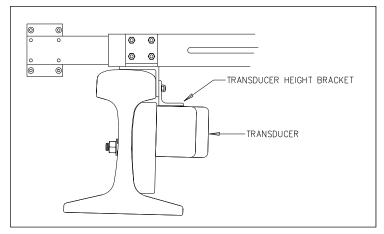
The fixture should be snug against the top and gauge of both rails. This may be impossible if the transducer body is less than 1-9/16 inches (3.97 centimeters) below the top of the rail <u>or</u> if the transducer body isn't parallel to the top of the rail.
