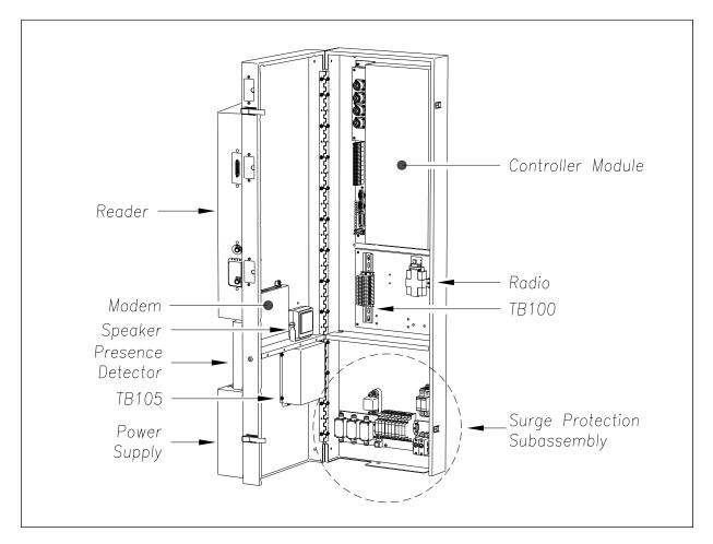
The SmartScanIS enclosure consists of two formed sheet-metal box panels that are joined by a continuous hinge and coated with a white polyester powder coat to provide a long-lasting finish. An enclosure can easily fit in a 4-foot x 4-foot signal bungalow. It is secured to a plywood backboard with six  $1/4 \times 1$ -inch lag screws. System modules are mounted inside and outside of the enclosure to reduce the size of the complete system.
