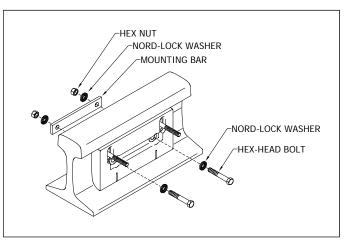
18 Tighten each hex-lock nut with a 9/16-inch torque wrench to a torque of 12 to 15 foot-pounds (16.3 to 20.3 newton-meters).
