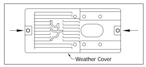
The **<u>type3</u>** wheel scanner has six. <u>Four</u> that attach the weather cover to the mounting plate and <u>two</u> that attach the mounting plate to the mount.
