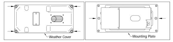
4 Separate the wheel scanner cover-and-module assembly from its mount.
