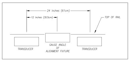
The fixture should be snug against the top and gauge of both rails.
