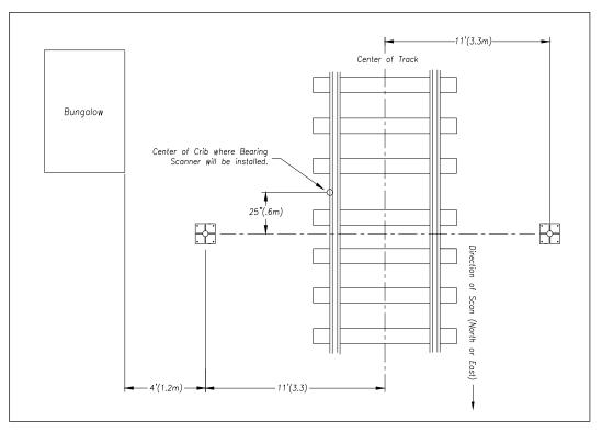
2 Lower one metal mast base into each hole, rotating it until one edge of the base is parallel to the track.
