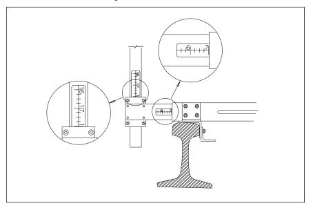
**13** Extend the vertical alignment bar to 18 inches  $\pm 1$  inch on the scale.
