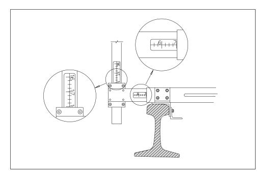
The fixture is used differently for bearing scanners and for wheel scanners. To align **type2/type3** bearing scanners, you use the optical system of the fixture. The key parts of this optical system are the target sight and the reflector block.
