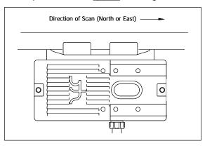
The top view of the **<u>type3</u>** bearing scanner mounting plate and weather cover are shown below.
