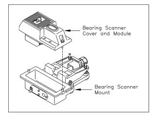
The figure below shows the major parts of a **type3** bearing scanner.
