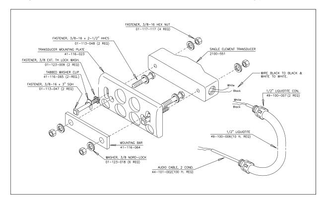
STC transducers consist of a horseshoe magnet with a tightly wound coil, encapsulated in a rigid epoxy potting compound. Each transducer is mounted 1-9/16 inches (3.97 centimeters) below the top of the rail. As the wheels of a railcar pass over the transducer, the wheel flange disturbs the flux field of the magnet, causing the output of a sinusoidal waveform of varying amplitude. The depth of the flange and the speed at which the wheel is moving determines amplitude.
