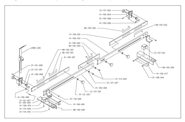
The figure below shows the parts of an alignment fixture (2066-000).
