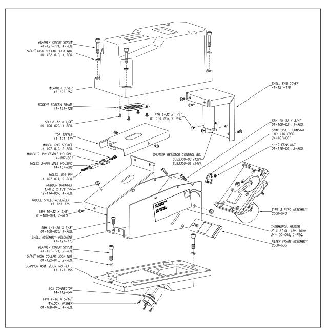
The figure below shows the parts of a <u>type3</u> bearing scanner cover-and-module assembly (2500-524**AC**). The <u>type3</u> bearing scanner uses a **black filter frame**.
