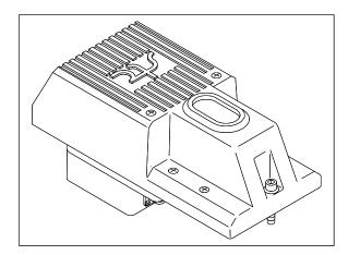
The figure below shows an assembled **<u>type3</u>** bearing scanner cover and module.
