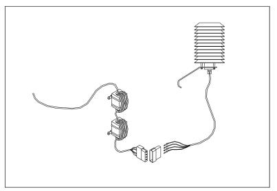
7 Using a wire stripper, remove 1/4 inches (6.4 millimeters) of insulation from the ends of the four wires coming from the other end of the RF-filter assembly.
