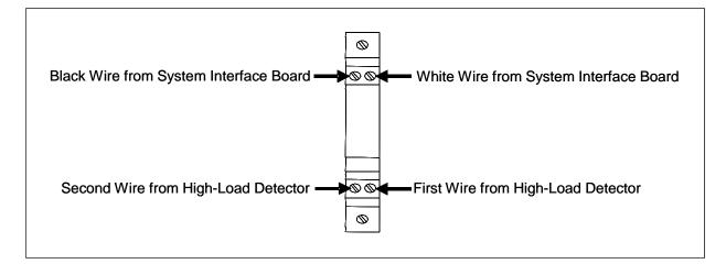
Correct polarity <u>need not be</u> observed when connecting the wires from the high-load detector. One wire from the detector should be connected directly below the existing white wire at row two of the UTB, and the other wire should be connected directly below the existing black wire at row two of the UTB.
