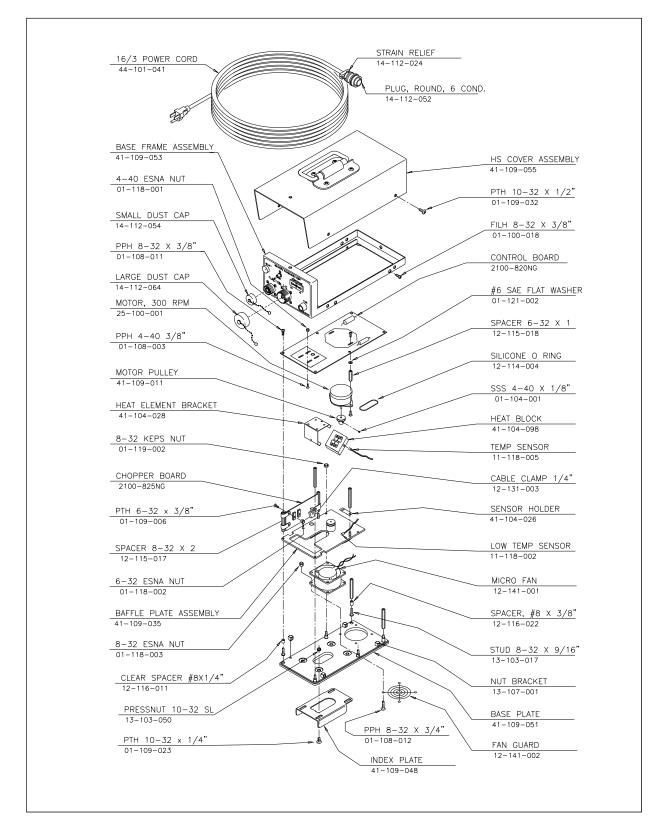
The figure below shows the parts of a calibrated heat source (2100-810NG).
