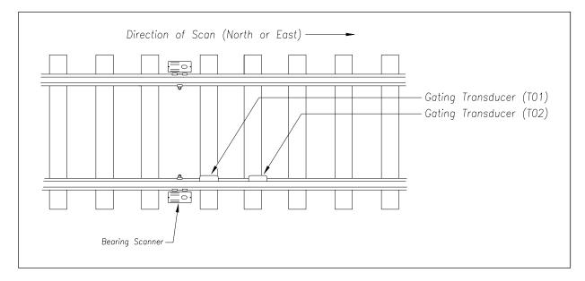
The **type2** bearing scanners are aligned to scan the bottom 3.5 inches (8.9 centimeters) of the bearing housing, about 7.25 inches (18.4 centimeters) from the gauge line.
