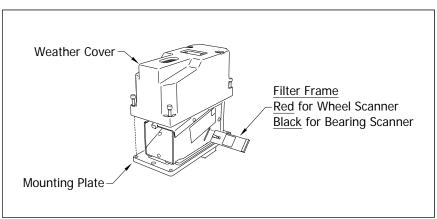
You'll need to remove the weather cover before you can check the color of the filter frame. Four socket-head-cap screws attach the weather cover to the mounting plate. Before continuing, be sure that the <u>black</u> filter frame is securely in place and that the four socket-head-cap screws on the weather cover are completely tight.
