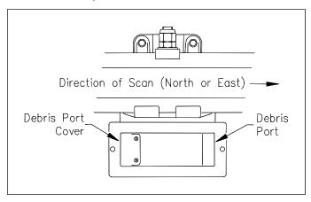
In the bottom of the mount are two rectangular holes called debris ports. One port is covered. One isn't. Do the next step only if the <u>uncovered</u> debris port is at the southmost or westmost end of the mount.
