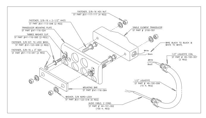
2100-550 Single Element Transducer - Exploded View
